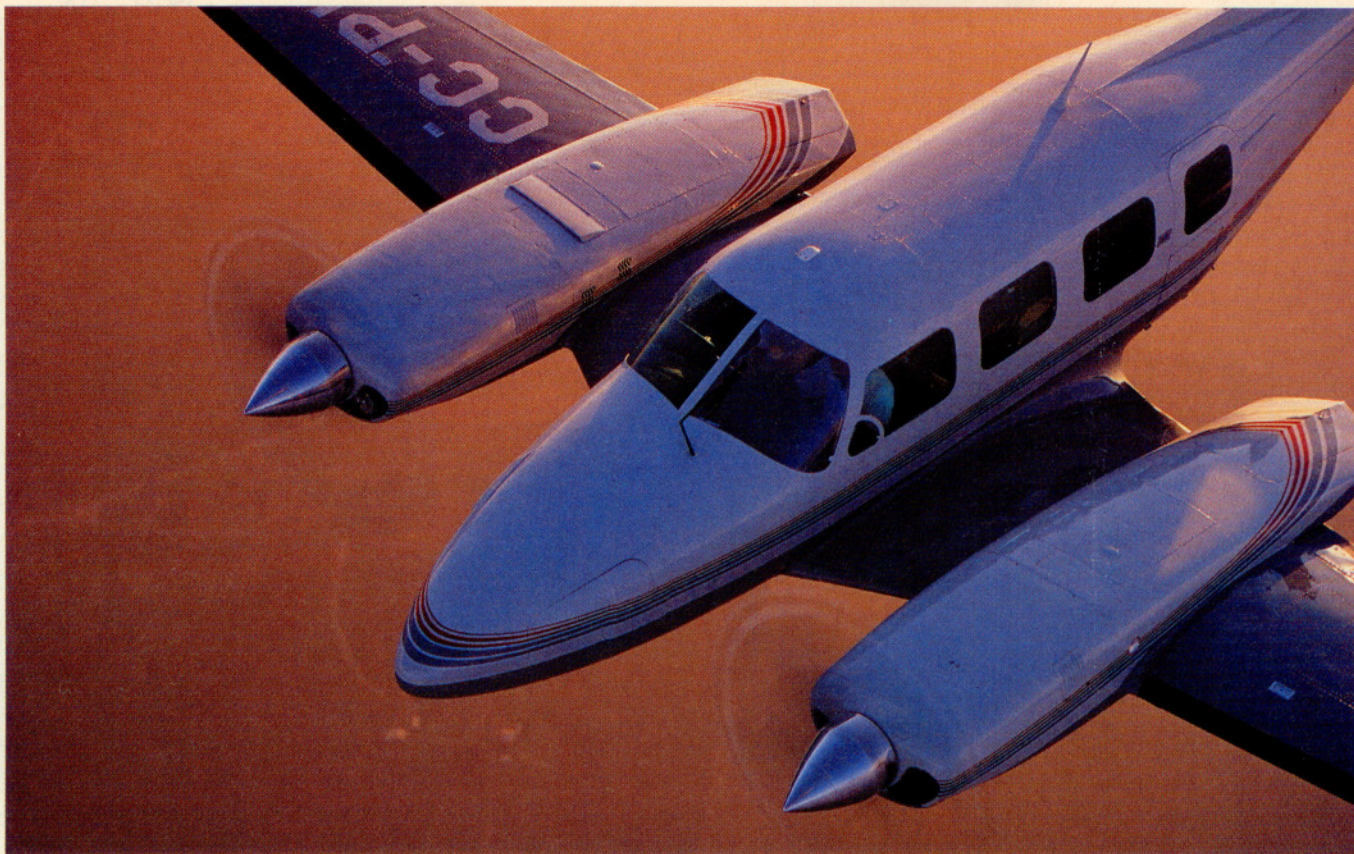
Colemill estimates that the Panther conversion provides a 10-percent increase in performance across the board. The redesigned cowl inlets (below) allow Panther owners to take off with the cowl flaps closed, boosting single-engine climb rate by about 50 feet per minute.
